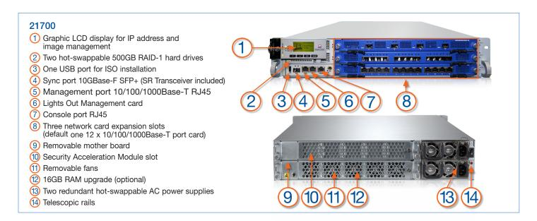
Furthermore, the 21700 also has a slot for an optional Security Acceleration Module. In addition to hot-swappable redundant disk drives and power supply units, the 21700 appliance also supports Lights-Out-Management (LOM) for remote support and maintenance capabilities. The 21700 Appliance is a highly serviceable chassis. Access to all components is easily available from the front and the back of the unit when mounted in the rack.
